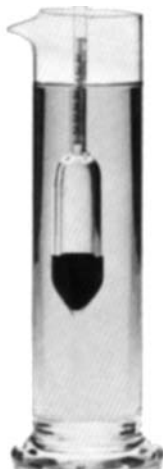
Plate 6.5 Urinometer for measuring urine mass density (specific gravity).
