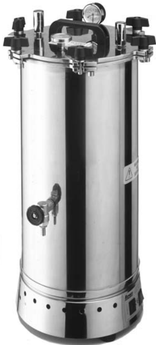
Plate 4.12 Dixon electric 2 kW heater autoclave of 30 litre capacity, model ST 3028, operating at 121 °C with temperature control and automatic cut-out. Courtesy of Dixon Surgical Instruments.
