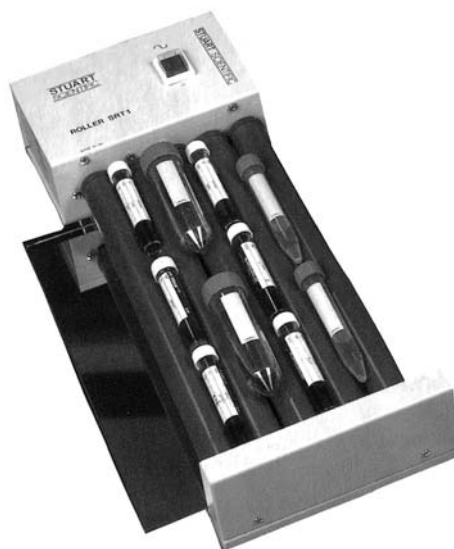
Plate 4.20 SRTI Stuart five-roller mixer that rotates and tilts specimens. Courtesy of Bibby Sterilin.
