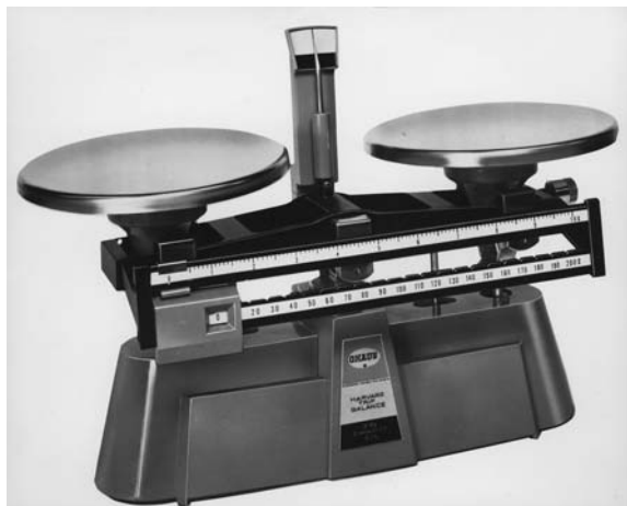
Plate 4.6 Ohaus Havard mechanical trip balance with readability of 0.1 g and capacity of 2 000 g.
